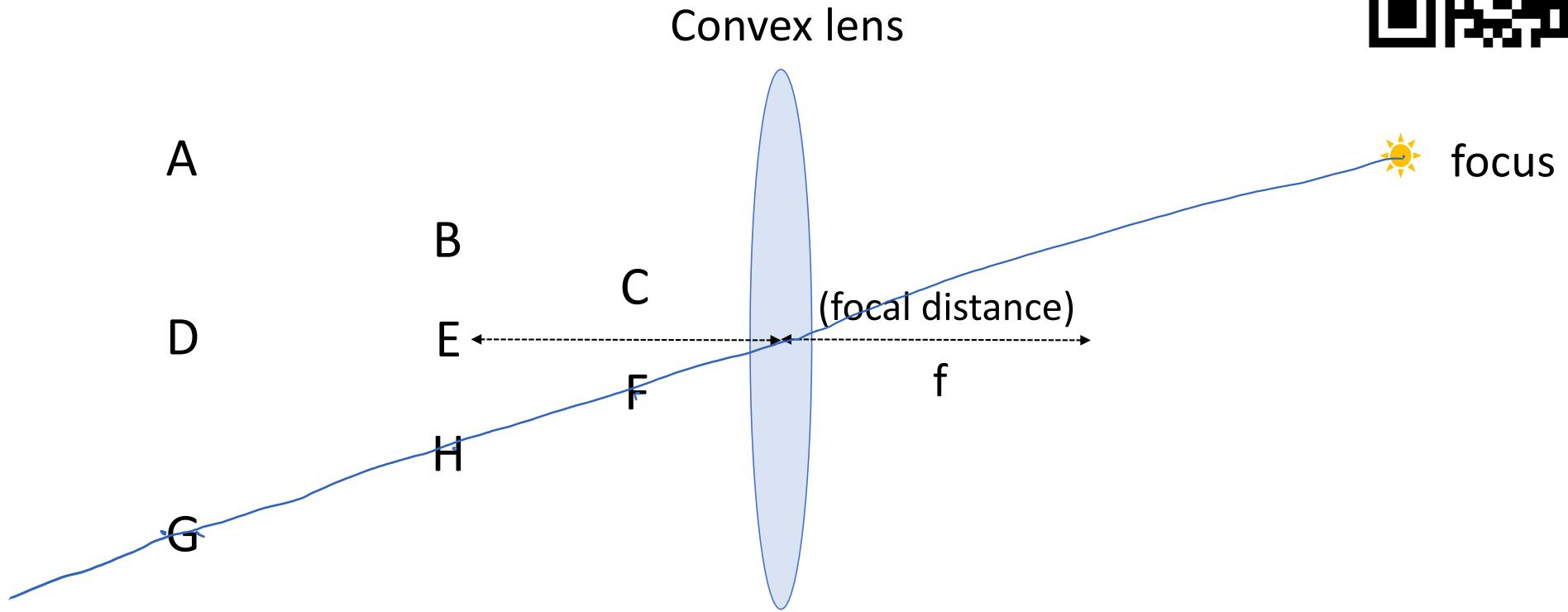
Thin lens equation :  $\frac{1}{f} = \frac{1}{d_o} + \frac{1}{d_i}$   $\xleftarrow{\text{OK}}$   $d_o = d_i = 2f$
