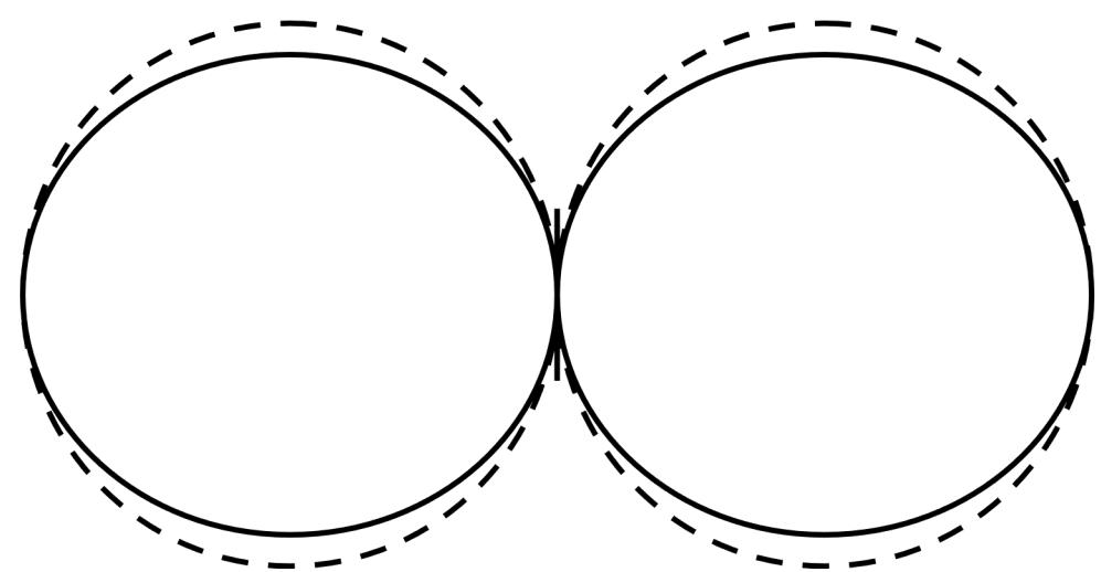
Radiation pattern of the short dipole (dashed line) compared to the half-wave dipole (solid line)
